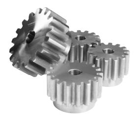
Silverthin<sup>™</sup> is pleased to offer standard, high quality mating pinions from stock for our ST and SK series slewing ring bearings. These pinions are made to AISI 4140 steel and are hardened to have a surface hardness of 55-60 HRC. See below for dimensional data.
